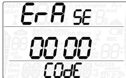
Nemo Wide allows you to reset the desaturation in the computer. Any tissue saturation information from a recent dive will be reset to zero and the computer treats the next dive as a non-repetitive dive. This is useful when the computer is loaned to another diver who has not dived in the last 24 hours.
