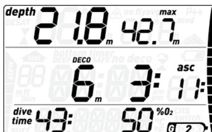
If you press the **+** button while G2 is blinking, the next available gas in the list will be displayed instead. This will be G1 if only two gases are set or if you are deeper than the MOD of G3, or G3 if you have set three gases and are shallower than the MOD of G3. Alternatively you can press **esc** to cancel the gas switch and stick with G1.
