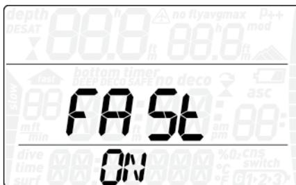
A fast (uncontrolled) ascent is defined as one in which a speed of 12 m/min / 40ft/min or higher was maintained over more than two thirds of the way up. This applies to dives deeper than 12m/40ft only. In such an event, due to the potential of harmful bubble formation, Nemo Wide locks the computer for 24 hours in order to discourage you from diving again. In this menu, you have the option to disable the locking up of the computer in the event of an uncontrolled ascent.
