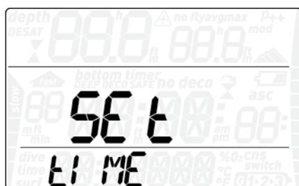
Press the **enter** button to enter a menu, press the **+** or **-** button to scroll up and down between available options or to increase or decrease the value of a setting. Then press the **enter** button to confirm the change in setting. Press the **esc** button to go up one level in the menu tree.
