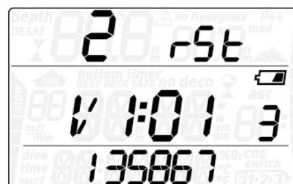
This submenu provides information about the hardware and software of your Nemo Wide and about the status of the battery with a number from 1 to 3, 3 being the highest, 2 corresponding to a steady battery symbol and 1 to the blinking battery symbol (no dive).
