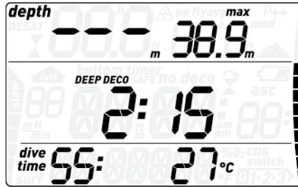
Upon returning to the surface, Nemo Wide first goes into the so-called surfacing mode. This mode allows you to resume your dive after a brief period of orientation. The screen shows a 3-minute countdown.
