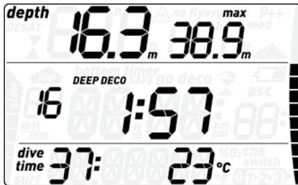
For DECO stops, since the duration is a function of the exact depth, only the minutes are shown.
