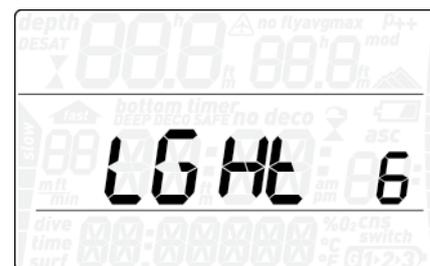
Nemo Wide has a backlight which can be activated in case of low ambient light. The backlight is activated by pressing and holding the **+** button. During a dive, the backlight will stay on for the duration defined in this menu. You can choose between 1 and 10 seconds, or you can set it to **on**. If you set it to **on**, the backlight will remain on until you press and hold the **+** button again.
