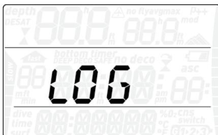
Nemo Wide can record the profiles of approximately 35 hours of diving, at a sampling rate of 5 seconds. The information can be transferred using the optional USB clip to PC via the Dive Organizer software or to a Mac via the Divers' Diary software. In addition, Nemo Wide can show most of the information directly on the display.
