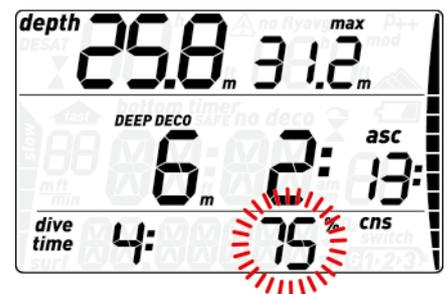
When the oxygen toxicity level approaches 100%. The alarm message and the audible signal are repeated for 5 seconds in one-minute intervals after the first occurrence and for as long as the value of CNS stays at or above 100%. Consider terminating the dive immediately!
