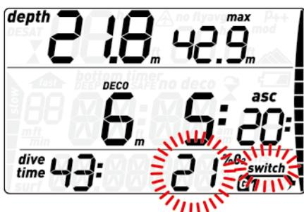
Press the **+** button while this indication is blinking to initiate the gas switch: the oxygen percentage of G2 starts to blink in lieu of that of G1, and in the top right corner the MOD of G2 is displayed, also blinking.
