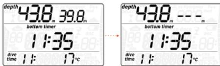
From any display, pressing the **enter** button restarts the stopwatch.
