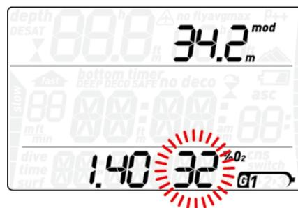
Once inside this menu, press the **+** or **-** button to change the O<sub>2</sub>% and observe how this affects the maximum operating depth (MOD). Then press the **enter** button to move on to the ppO<sub>2</sub>max and use the **+** or **-** button to change the value, again noticing how this affects the MOD. Press the **enter** button again to save the setting.
