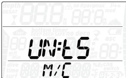
You can choose between metric (depth in meters, temperature in °C) and imperial units. (depth in feet, temperature in °F).
