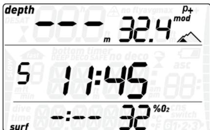
The pre-dive display shows p factor and altitude settings, time of day, surface interval since the last dive and temperature. If Nitrox is set, it will show the O<sub>2</sub> percentage and the corresponding MOD. A small S or F to the left of the middle row indicates the water type.
