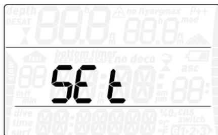
Nemo Wide's **SEt** menu allows you to change settings. Once inside this menu, press the **+** or **-** button to scroll between two submenus: **SEt dIVE**, where you can set parameters pertaining to the dive, and **SEt tIME**, where you can set parameters pertaining to time and date.
