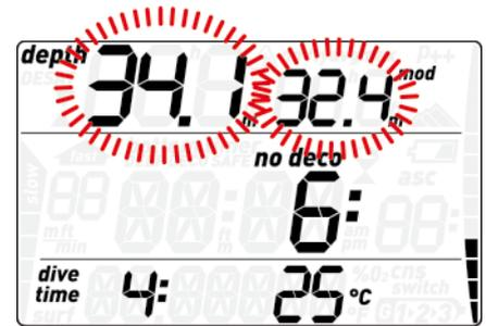
The alarm persists until the diver has ascended enough for the  $ppO_2$  to return within the set limit.
