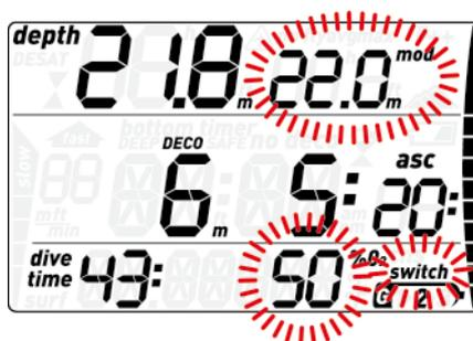
Press or press and hold the **enter** button to confirm the switch to G2: the set oxygen concentration will be displayed steadily in the lower right corner of the screen, and within 20 seconds the ascent time is updated to reflect the higher oxygen concentration in the breathing gas.
