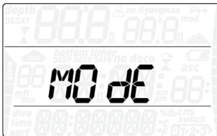
Here you can define the type of gas you will be breathing during the dive (air or enriched air nitrox, including multigas). You can also set Nemo Wide to bottom timer, in which case Nemo Wide will show only time, depth and temperature: it will not carry out any decompression calculation and it will not show any warnings and alarms.
